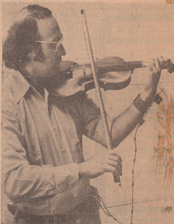
Burton Kaplan demonstrating one of his Practice Partners, strapped to his arm. If he moves his hand incorrectly, the buzzer on his belt sounds. The buzzer is attached by a wire to the device on his arm.
